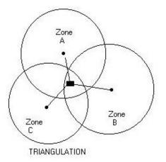
The small black box in the above pic indicates your vehicle, you can see that it is nearer zoneA, and zone C, although Zone B has detected it, it is further away
