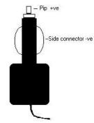
Site the tracker unit out of site but where it will not be subject to excessive vibration, or where moisture may get into the unit. Also as far away as possible from things like alternators, indicator relays, electronic ignition units, and other sources of possible RF interference.
